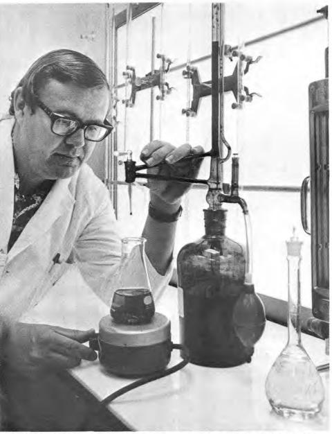
CHARLES GRAY (3311) runs through a titration technique for determining toxic gasses in an air sample. Charles is currently revising the handbook used as a reference in the analysis of laboratory samples.
